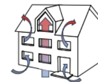
How radon enters the house - Stack Effect
