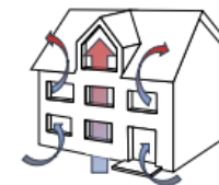
How radon enters the house - Stack Effect
